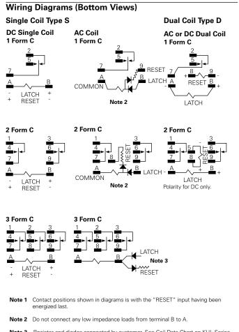
**Note 3** Resistor and diodes connected by customer. See Coil Data Chart on KUL Series engineering data page for resistor value. Recommended using 1N4007 diode.
